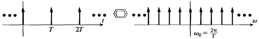
Figure 6.7 The Fourier transform of a “picket fence” time signal with spikes separated by T is a “picket fence” frequency spectrum with spikes separated by \omega_0 = 2\pi/T .
