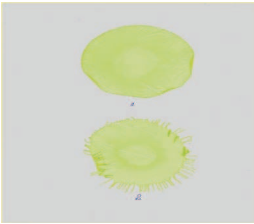
Fig. 2 Picture of dendrimer membrane with covalently immobilized fluorescent dye and enzyme
