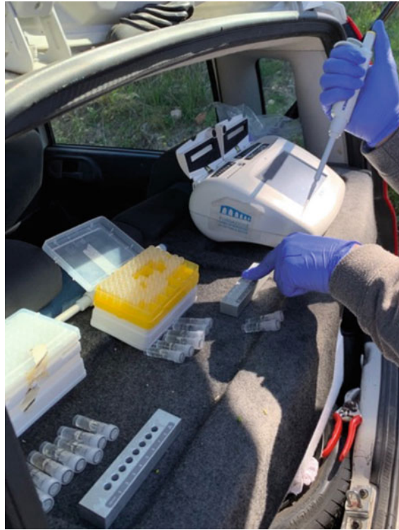
Fig. 3 Xylella fastidiosa field diagnosis by using real-time portable LAMP instrument (Genie II, OptiGene)
