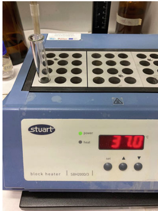
Fig. 2 Samples are dried at 37 °C under nitrogen atmosphere
