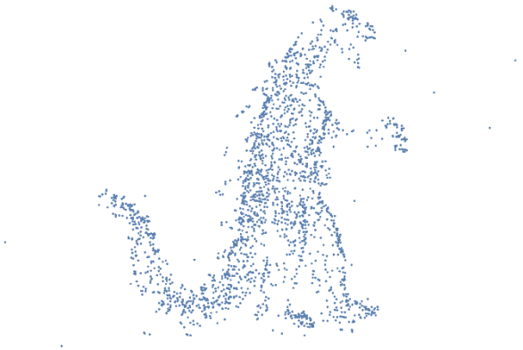
Fig. 13.4: The 4983 3D points that have been triangulated from the dinosaur data set in Example 13.5.
