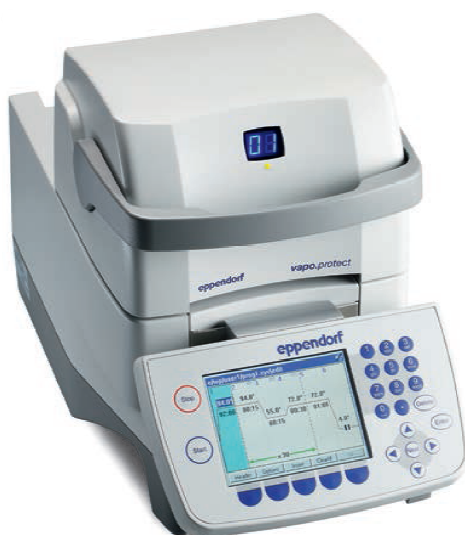
Figure (11.22). PCR thermocycler for gene amplification (manufactured by Eppendorf – Germany). This machine is lovely designed for the every researcher where it can be controlled by touching directly on its screen.
