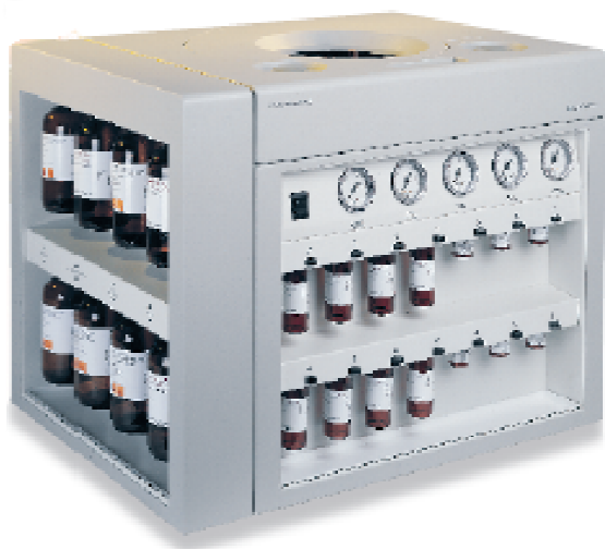
Figure (11.6). DNA synthesis machine. It's possible through this machine to synthesize different DNA sequences according to the purpose of research, such as PCR primers, genes ... etc. (this device is from Applied Biosystems – USA).
