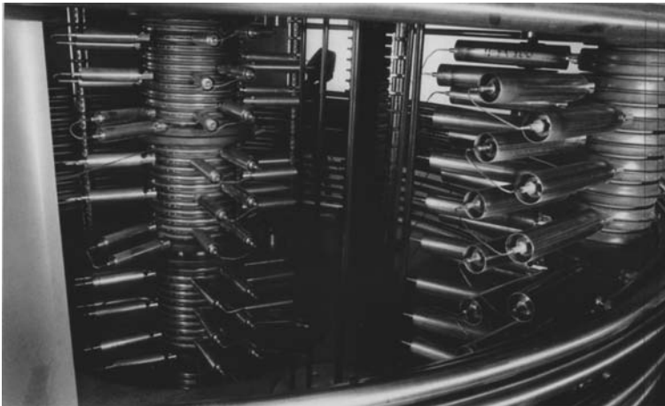
Fig. 7.9. The compact column and tube resistors in the ANU Pelletron
