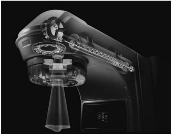
Fig. 2.3. A linac for radiotherapy equipped with a multileaf collimator. The electron beam is bent in a 270^\circ magnet. After flattening and collimation, the electron beam can be used for treatment. In most cases, however, the electron beam collides with a heavy-metal target, and the high-energy bremsstrahlung produced is used for treatment after flattening and collimation with the multileaf collimator (Reprinted with permission from Varian Medical Systems Inc.)
