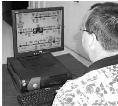
Fig. 16.2. A satellite computer used to control the High Voltage Engineering Corporation model FN tandem accelerator and associated components at the Center for Accelerator Mass Spectrometry, Lawrence Livermore National Laboratory. Essentially the entire accelerator system can be controlled from a single computer screen. Photo courtesy of William Fields, CAMS, LLNL
