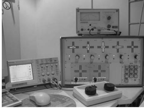
Fig. 15.6. Beam diagnostic equipment at the Rossendorf 3 MV Tandetron: beam position monitoring by slit devices and LED display ( center ), NEC beam profile monitor ( left ), current measurement using retractable FC ( top ), and computer-controlled parameter variation ( foreground )
