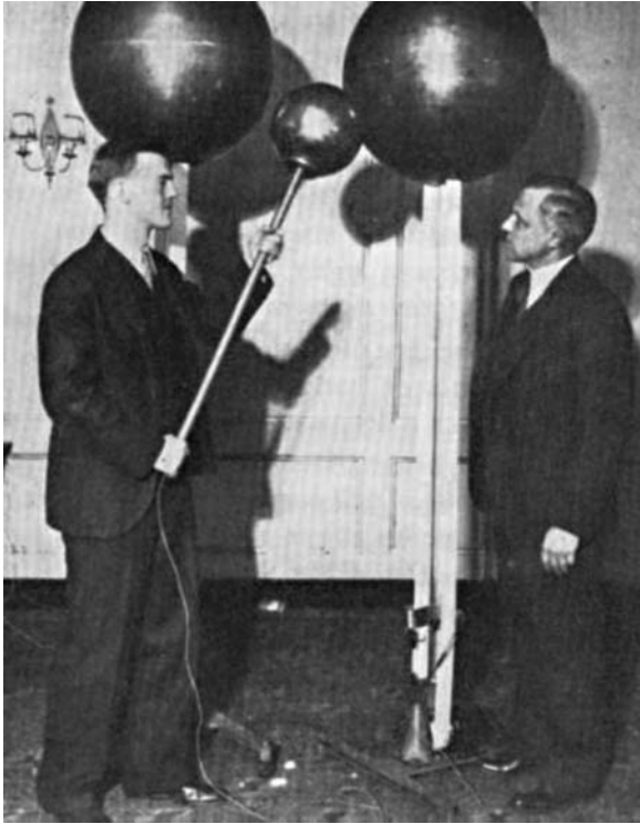
Fig. 1.2. Robert Van de Graaff ( on the left ) and Karl Compton in 1931. This test generator was a double unit consisting of positive and negative hollow spheres mounted upon upright Pyrex rods. Each sphere was charged by a silk ribbon belt, running from a grounded motor pulley at the base of the rod to a pulley in the interior of the sphere. Intersphere voltages of 1.5 MV were reported from this simple machine (Reprinted from [5], copyright 1974, with permission from Elsevier)
