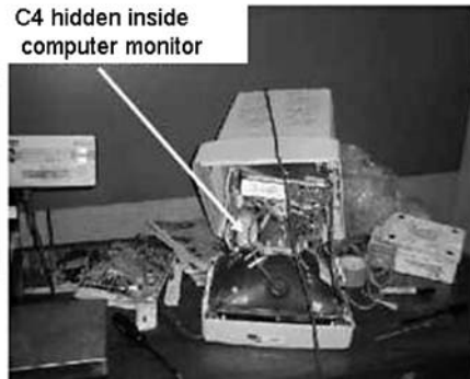
Fig. 22.7. Test results: PFNA inspection of an air cargo container loaded with computer monitors with a small concealed piece of explosive
