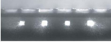
Figure 7.16: Crosssection of a printed circuit board with four waveguides in the optical layer illuminated by VCSELs (photograph courtesy of E. Griesse, Universität Siegen, Germany).
