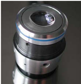
Figure 13.4: Photograph of a Zeiss objective lens for inspection microscopes. The objective lens contains an interferometrically fabricated diffractive optical element for achromatisation (specifications: working distance: 7.8 mm, NA = 0.65, cement-free assembly). (photograph courtesy of Dr. R. Brunner, Carl Zeiss, Inc., Jena).
